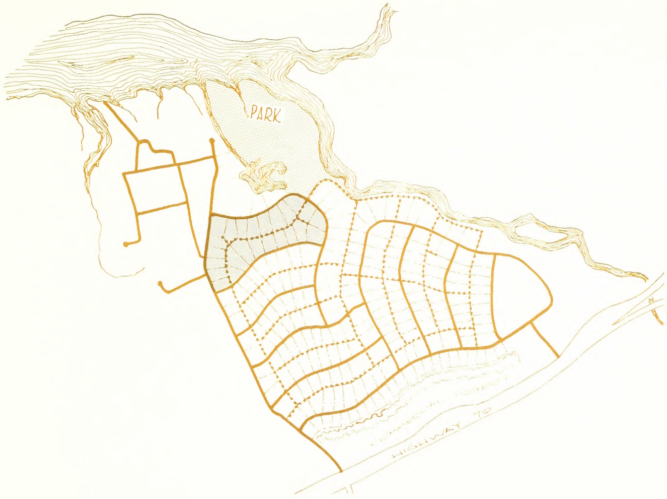
Back yard set-backs provide for the movement of people separate from the movement of cars
